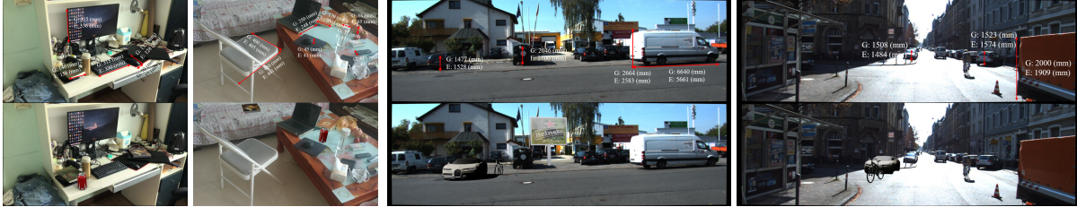
Figure 1: Scale-aware insertion of virtual objects into videos. Top: Input frames with extracted dimension and optimized size information of objects in videos ('G' for the ground-truth sizes, and 'E' for the estimated sizes). The red lines indicate the extracted plausible dimensions of the objects. Bottom: Output frames with different objects inserted with proper sizes.
