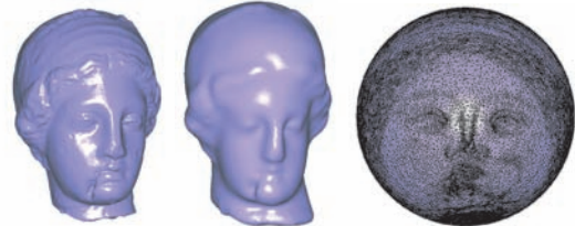
Figure 5: Updating the geometry via modifying curvature field. (left) Input model, (middle) non-shrinking smoothing, (right) spherical mapping.
