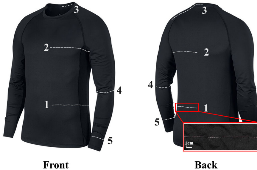
Figure 5: The placement of sensors on a garment according to anthropometry. The bottom right image shows one sensor after being sewed to the garment.
