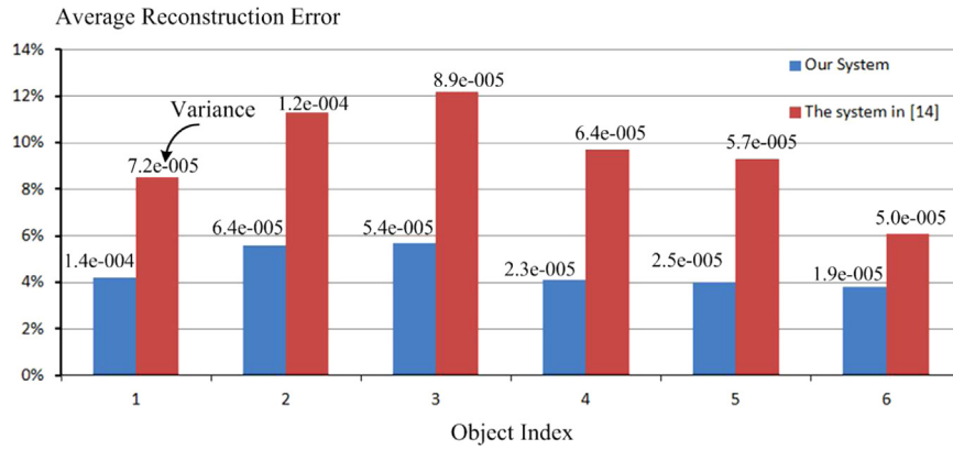
Fig. 5. Mean and variance of reconstruction errors measured using Eq. (12) for each object in six test scenes. Note that scene index 1 corresponds to the scene in Fig. 1 and scene indexes 2–6 correspond to the scenes in Fig. 6(1)–(5).
