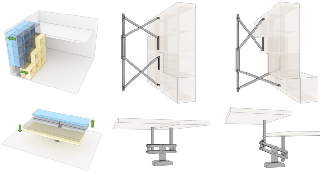
Fig. 18. Two examples show the usage of linkage mechanisms that drive a pair of boards in opposite directions simultaneously.
