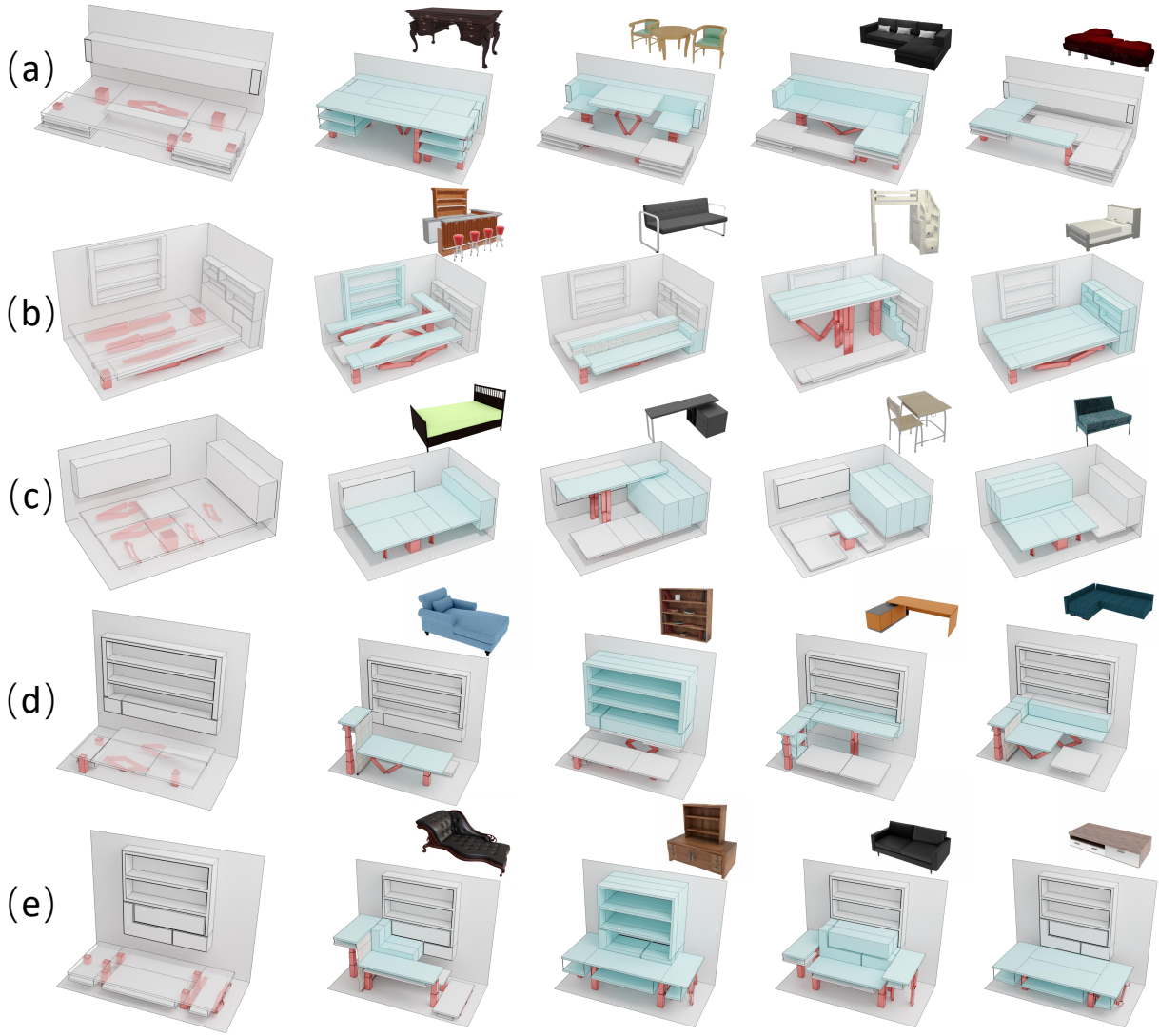
Fig. 10. Galleries of the designed multi-function furniture objects by our system. In each row, we show the folded state of the furniture (Left), four reconfigurations, and their associated reference furniture. The parts that participate in the reconfiguration are highlighted in blue.
