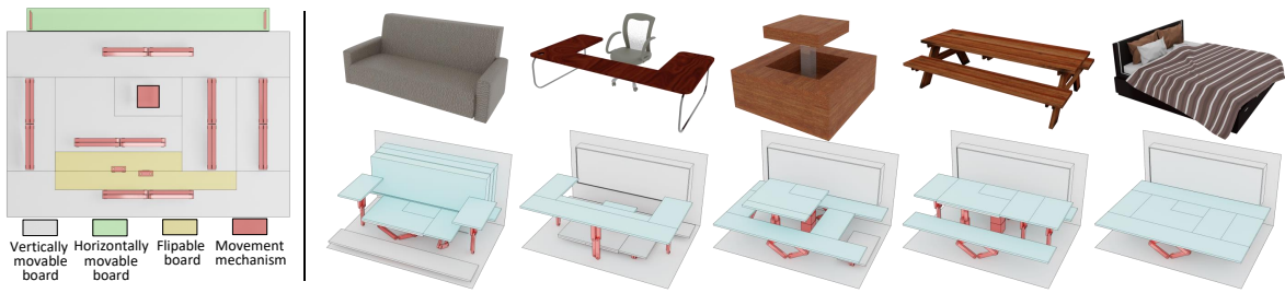
Fig. 2. An example of the multi-function assembly designed by our Magic Furniture system. Left: the 2D projection of such a design with movable boards and movement mechanisms. Right: the input reference shapes (Top) and the associated reconfiguration (Bottom), which consists of certain movable boards (highlighted in blue), to support multiple functions with a space-saving design.
