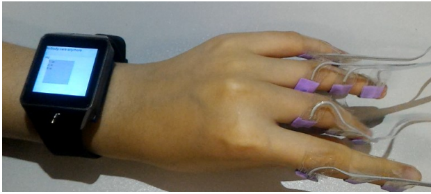
Figure 2: Experimental prototype of FingerT9 .
