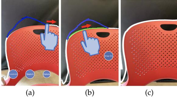
Fig. 13. 2D sketching. The user selects a curve segment (in blue in (a)), and draws a desired 2D curve (in green in (b)) in a frozen view. Edge snapping is used in (b) to help create accurate curves. The blue hand icon and the red arrow are added to the figure to illustrate the gesture interaction.
