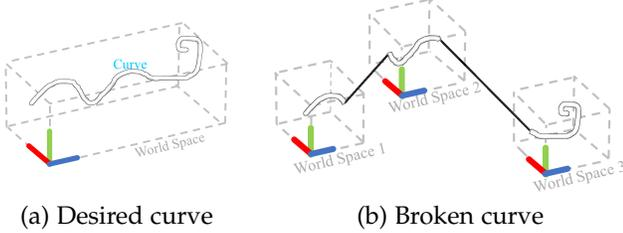
Fig. 6. A world coordinate system might be re-estimated due to the sudden track loss, which breaks a desired curve.
