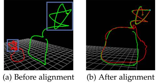
Fig. 8. (a) The curves generated by ARKit and MoCap were not aligned. (b) We used the corners of a specific shape (in purple box) to align the curves.
